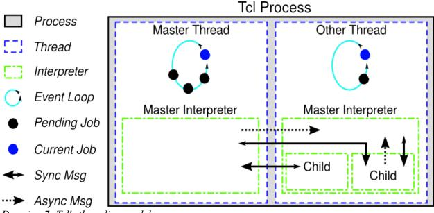
Drawing 7: Tcl's threading model.
