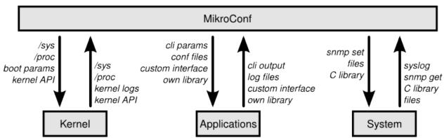
Drawing 1: Set/Get mechanisms MikroConf uses to interact with its software environment.
